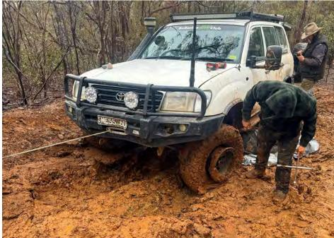
second tyre off it's bead, with a gouge in the side and a broken axle, we made it to the top of the first hill.
